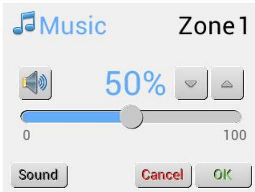
The slider or the up/down buttons can be used to change the music volume (in %). Be sure to have a proper input signal range (see section 4.6.1)
