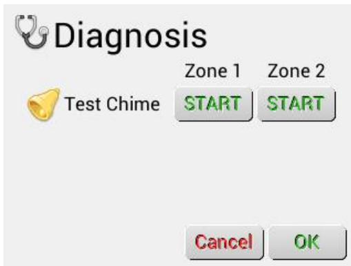
Click on Start button to generate a chime test signal to help to determine the location of the speakers in each zone.
