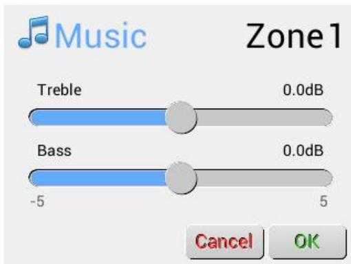
The Treble/Bass sliders are used to make the EQ adjustments on the music output.
